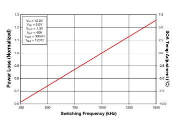
Figure 6 Normalized Power Loss vs. Switching Frequency
