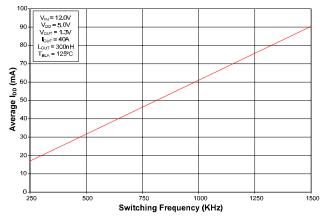
Figure 7  $V_{DD}$  Supply Current vs. Switching Frequency
