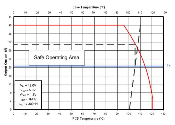
Figure 10 SOA Example, Continuous current  $\approx$  31A for T<sub>PCB</sub> = 100°C & T<sub>CASE</sub> = 110°C
