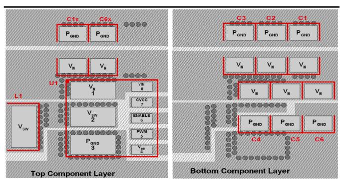
Figure 13 Top & Bottom Component and Via Placement (Topside, Transparent view down)
