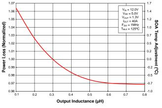
Figure 5 Normalized Power Loss vs. Inductance
