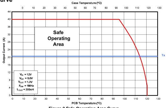
Figure 2 Safe Operating Area Curve
